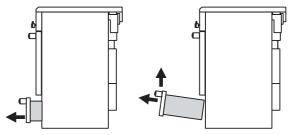
Your installer may not have left the levelling tool in place. If not, locate it as shown. If you cannot find the levelling tool, contact your installer.
